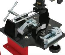
This Putter Bending Gauge was designed for retail shops and clubmakers who wish to set up a fast turnaround putter fitting system, where ease-ofuse, speed, and accuracy are all important. Bending bars not included
