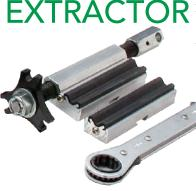
Accommodates all shaft sizes. Secure the shaft between the Shaft Extractor pads with the hosel positioned in the appropriate holder. Attach the ratchet to the other side, apply heat and glide the head off the shaft tip! A constant 4" of clamp pressure prevents slippage.
