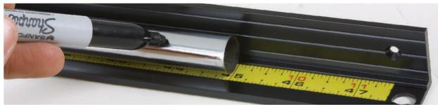
Everything you need to know for proper shaft trimming is included on pages 74-75. Each shaft in this catalog has a Shaft Trim Code listed. Consult the chart on page 75 to determine how much to trim off the shaft. **Unless noted, all directions are for TIP trimming. After tip** for each of the manufacturers. trimming, trim to playing length from the butt.
